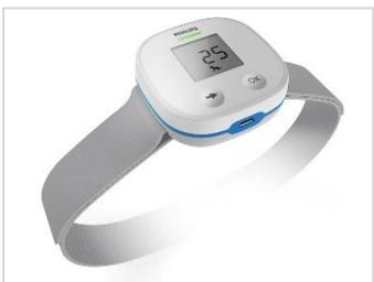
The Philips Children's Automated Respiration Monitor (ChARM) converts chest movements detected by accelerometers into an accurate breathing count, using specially developed algorithms. The device not only provides quantitative feedback, but also qualitative feedback to the healthcare
