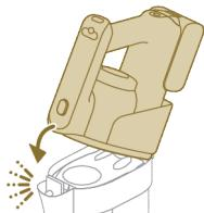
5 Reconnect the 3-in-1 handheld to the dust bucket. Make sure that you connect the rear part first, then connect the front part so it locks into place with a click.
