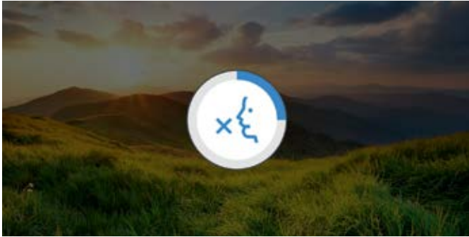
The breath-hold guidance function coaches patients through the breath holding that is needed for some scans. It shows a patient when to start and how long he or she still needs to hold breath.
