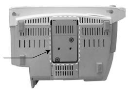
1. Fasten the Philips-supplied Table Top Mount to the Mounting Adapter (front end of Arm) with one (1) M6 x 12mm FHMS and two (2) M6 x 8mm FHMS.
