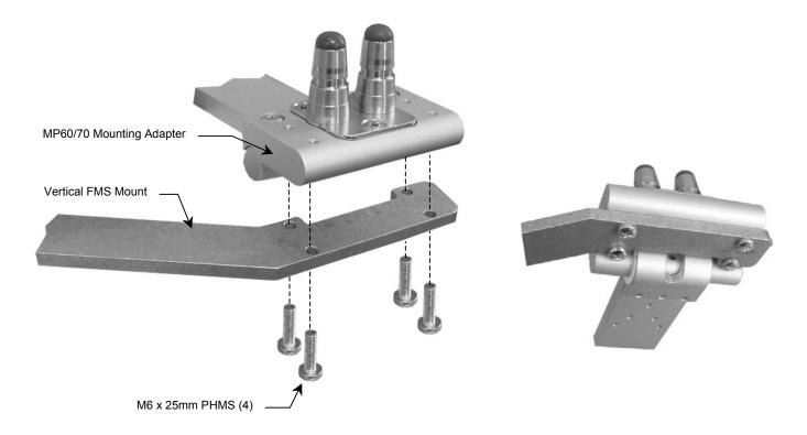
2. Clamp Flexible Module Server (FMS) to Vertical FMS Mount. It may be necessary to remove, rotate, and reattach the pole clamp at the rear of the FMS, to clamp it in a vertical orientation.
