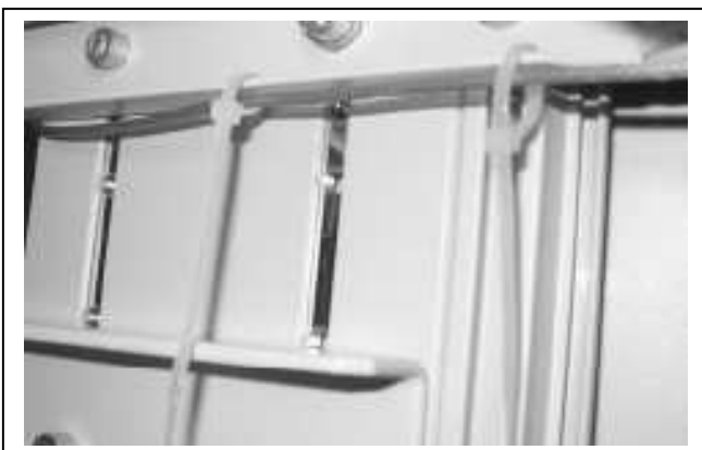
Fix antenna cable with cable winder
