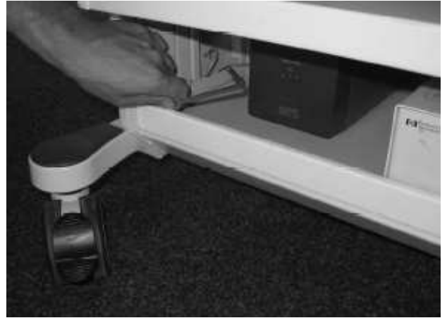
Mount bar after placing equipment
