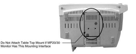
1. Fasten Table Top Mount to Mounting Adapter with one (1) M6 x 12mm FHMS and two (2) M6 x 8mm FHMS.
