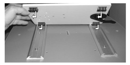
2. Lock the Camlock Plate by moving Camlock Lever from right to left.
