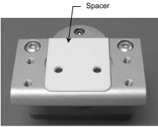
2. Using the 3/16" hex wrench, fasten the monitor to the Mounting Adapter with two (2) M6 x 16mm SHCS.
