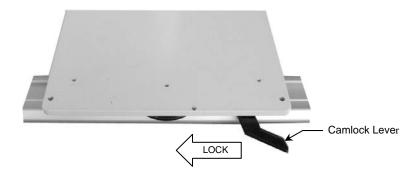
3. To prevent the Camlock Lever from being unlocked, insert one (1) #6-32 x 3/8" PHMS in the threaded hole to the right of the Lever (below right). To further secure the Camlock Mount in the Rails, insert one (1) M4 x 20mm PHMS in each of the two (2) threaded holes at the rear corners of the Mount (below right). Stop tightening these screws when they make contact with the bottom of the Rail.
