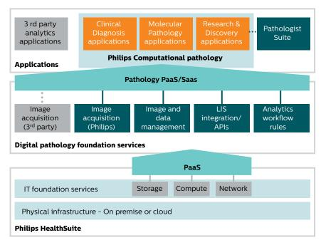
High level architecture of the Philips IntelliSite pathology solution as deployed on an IT platform. The IT services are provided to the pathology platform by a Platform as a Service (PaaS) style interface. The Pathologist Suite and other front-end applications can be consumed as a Software as a Service (SaaS).
