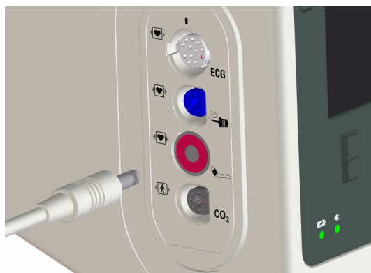
Figure 9 Connecting the NBP Cable
