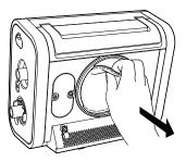
Place a new filter onto the bayonet mount then twist the filter clockwise a quarter of a turn while pressing in to secure.
