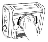
Replace the filter cover and turn clockwise to secure.
