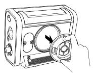
Twist the filter counterclockwise a quarter of a turn, and then pull straight out to remove.
