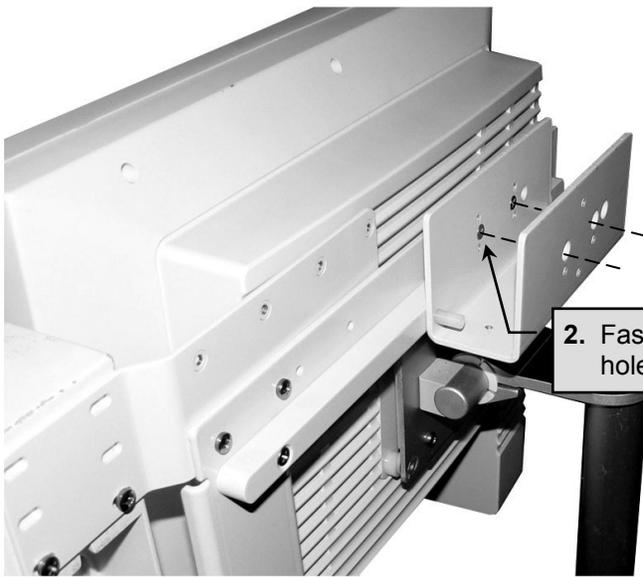
2. Fasten Power Supply Holster to two (2) mounting holes in the Remote Bracket as shown.
