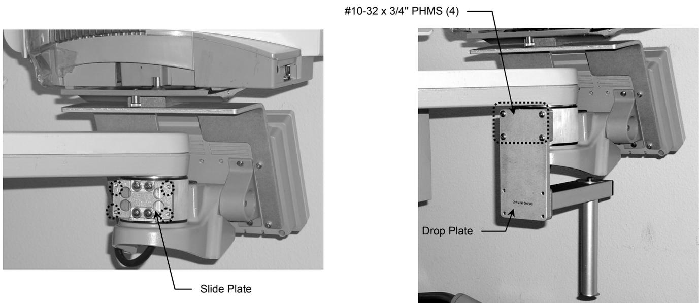
3. Clamp module rack (or other device with clamp) to the Post.
