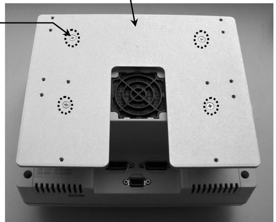
3. Locate four (4) threaded mounting holes on Subplate (below left). Using four (4) M4 x 8mm FHMS, fasten Subplate to display arm.
