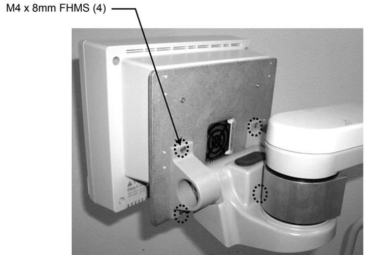
4. Locate four (4) mounting holes on Subplate (below left). Using four (4) M4 x 12mm PHMS, fasten Display Mounting Bracket to Subplate. **Installation Note:** An upper set of mounting holes is provided on Subplate if additional height is required for the patient monitor.
