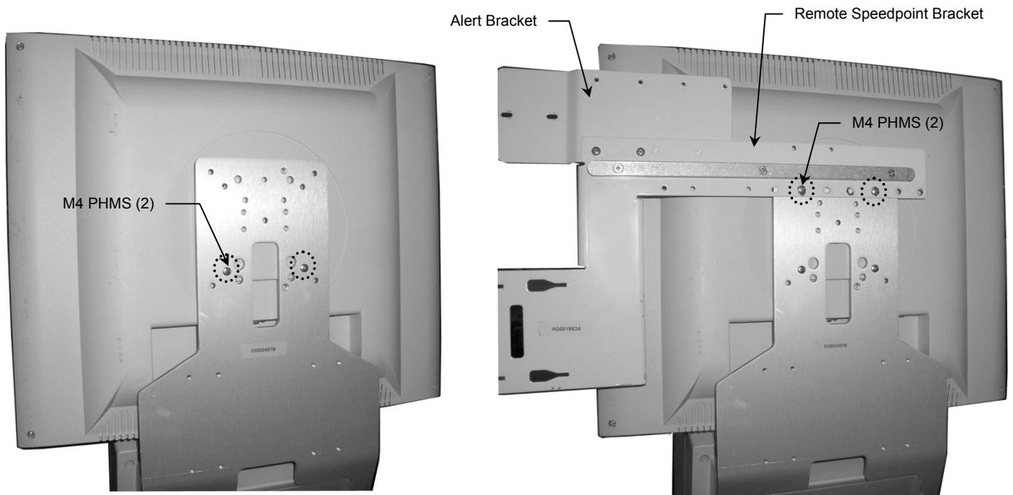
5. Complete bracket/instrument mounting in accordance with *Philips MP90 Remote Speedpoint Mounting Bracket and Adapter*, and *External Alert Device Mounting Bracket (DU-AG-0019-80)*.
