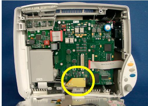
Old LG-Philips/3M Version - Remove Flex Panel Adapter Cable
