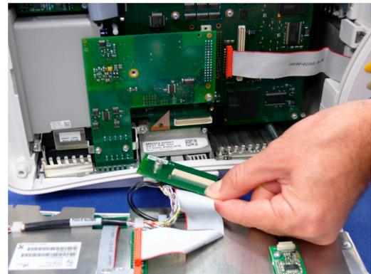
New Sharp/ELO Version - Remove Panel Adapter Board
