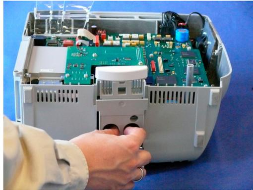
8 Insert the fix mount with the white release knob cover and secure it with two screws.
