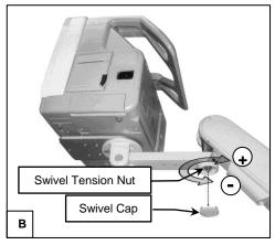
7.4 Rear Pivot Tension Adjustment – To adjust the tension at the rear Pivot Point (closest to channel), tighten (+) or loosen (-) the Pivot Tension Nut with a 3/4" or a 19 mm socket wrench until desired tension is achieved. Do not remove the Pivot Tension Nut.
