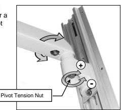
**7.5 Center Pivot Tension Adjustment (VHM-25 with Extension**)- Insert finger into the front of the Cable Cover and pull down to remove (Fig. A). Tighten (+) or loosen (-) the Pivot Tension Nut with a 3/4" or a 19 mm socket wrench until desired tension is achieved (Fig. B). Do not remove the Pivot Tension Nut. Push Cable Cover up into the Arm until the tabs on the side of the Cable Cover snap into place (Fig. C).
