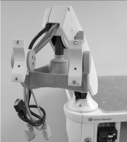
2. Using the 5 mm hex wrench provided, fasten the Mounting Bracket to the arm with four (4) M6 x 16 mm SHCS as shown.
