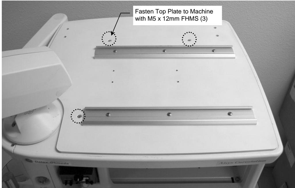
3. Unscrew and remove right and center screws from front Camlock Rail. Loosen left screw and rotate Rail enough to allow access to fourth mounting hole. Install M5 x 12mm FHMS in threaded insert. Return Rail to original mounting position, reinstall right and center screws, and tighten left screw in Camlock Rail.
