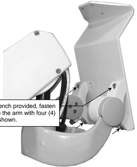
3. Thread four (4) M4 x 12mm SHCS into the mounting holes of the 75mm VESA mounting pattern on rear of ventilator display. Leave 8mm of thread exposed for inserting screw heads through keyholes in Mounting Bracket.
