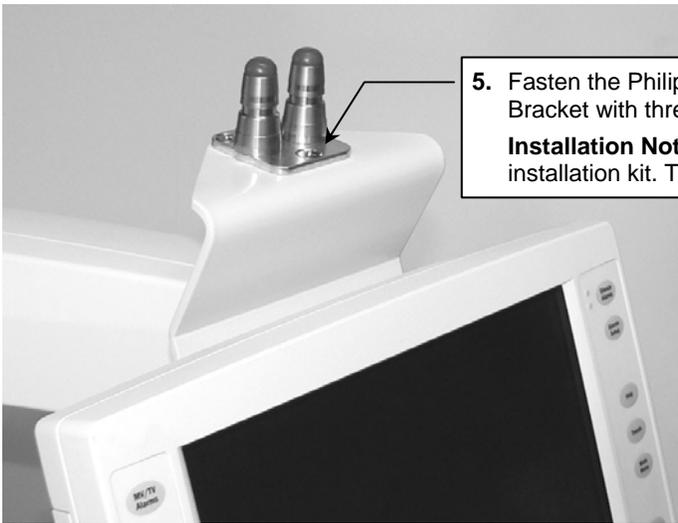
5. Fasten the Philips-supplied table top mount to the top of the Mounting Bracket with three (3) M6 x 8 mm FHMS.
