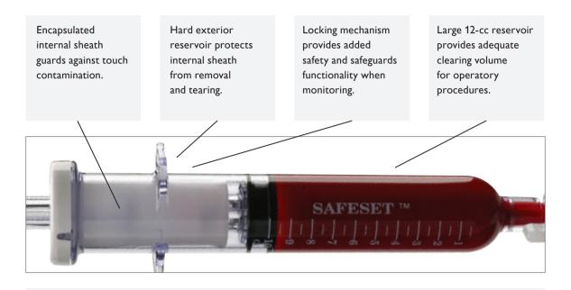
In-line reservoir provides a straight fluid path to minimize turbulence and maintain high waveform accuracy, and adds convenience for both drawing blood and flushing the system afterwards.
