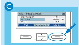
Navigate to **Circuit Type** and press Modify
