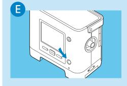
Press to begin therapy or continue navigating through the menu to set-up the ventilation parameters
