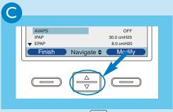
Scroll up and down using  $\frac{\Delta}{\forall}$  to navigate through the settings and alarms
