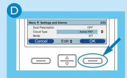
Use to choose **Active PAP** (exhalation valve set-up) or **Passive** (exhalation port set-up) and then press OK twice to confirm
