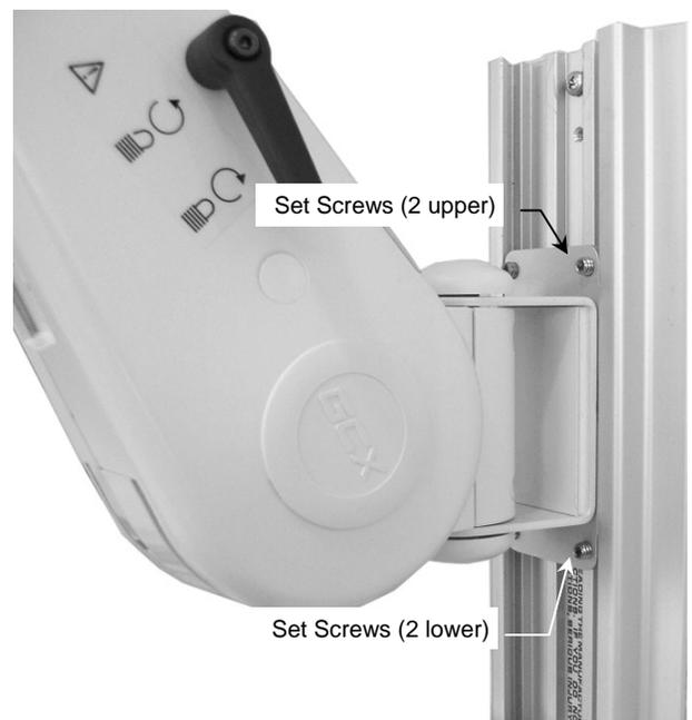
4. Mount the monitor in accordance with Philips Table Top Mount instructions. Attach Down Post if required (see procedure below) and proceed to "Counterbalance Adjustment" on page 4. **Installation Note:** Counterbalance Adjustment must be performed after monitor and FMS are mounted on the Arm.
