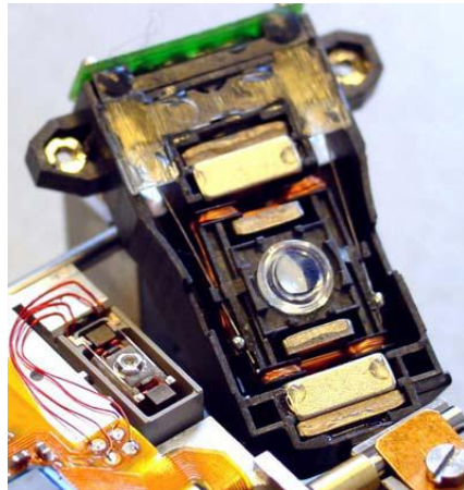
Figure 16. A tracking actuator from a DVD player
