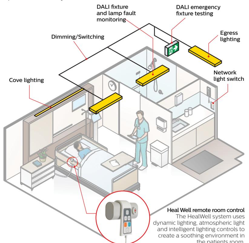
As well as providing an easy-to-operate user interface, Dyalite offers the flexibility for use in both new and retrofit applications. The system architecture allows the installer to add new sections without disrupting any elements of the existing lighting control infrastructure. This ability facilitates the organic growth of the lighting system over time without any detrimental effects to the day-to-day running of the hospital.
