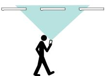
For proper commissioning, hold the phone above your head, pointed at the luminaire that you wish to target. This will help ensure that the IR range or cone is restricted to just one luminaire, and only that luminaire will react. Holding the phone closer to eye level or lower will result in a wider IR range or cone. This will cause multiple luminaires to receive the signal.
