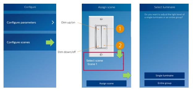
The scenes are selectable via the scene buttons of the switches associated either to the luminaire or an entire group. In any case, the configuration proceeds through the "Adjust light level" screen that enables the user to select desired light level for the selected scene.
