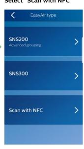
Place the back of the smartphone (where the NFC reader is located) onto the sensor NFC antenna (almost touching) to enable NFC communication. NFC communication might take a few seconds. Do not move until you hear a beep and the next screen appears.
