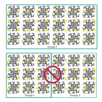
When configuring open plan offices with SpaceWise, large groups of 30-40 luminaires are recommended to maintain the lighting aesthetics of the space. Smaller groups may turn off more frequently than desired.
