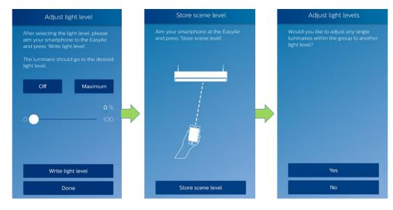
For a given scene, individual luminaires within the group can be configured to different light level settings. This is beneficial for example in a conference room where luminaires closer to the projection wall are desired to be dimmed/off while other luminaires in the same group are desired to be at higher light levels on the same scene.
