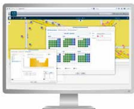
You get the flexibility to adapt every single luminaire to changing situations or demands of the city at any time. To adjust calendars to the individual needs you are free to change the “switching points” of every dimming profile simply via drag & drop.
