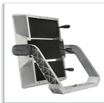
Rear view of BVP520 floodlight. Each light module is equipped with a ~10 cm cable with a quick connector plug at the end, making it easy to plug in the three cables from the external driver box.
