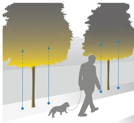
Luminaires with a wide beam are placed under the vegetation and aimed upward. The light makes the inside of the tree glow, revealing the volume of the crown.
