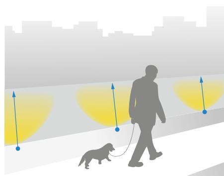
Lighting the vertical surfaces will act as visual guidance. A recessed floodlight will integrate perfectly with the surrounding by daytime. The frosted glass will diffuse the beam and create a subtle, soft effect.
