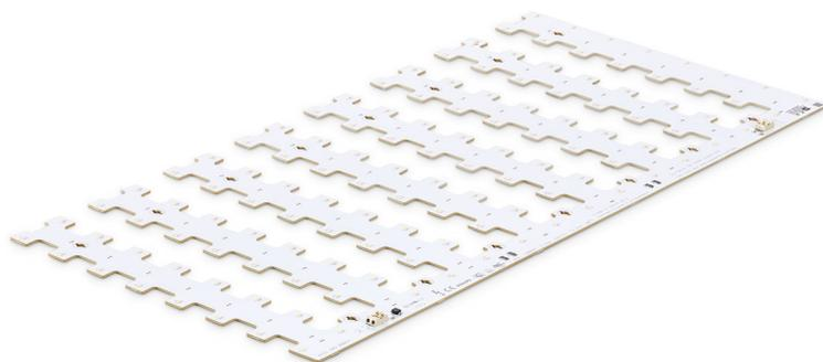
The Fortimo LED Square 2500 lm is a high performance solution offering best-in-class efficiency up to 175 lm/w. The rectangular square (260 x 520mm) is designed to reduce material and assembly cost for the OEM, compared to the 260 x 250mm design of the previous generation and many other brands. The footprint however is backwards compatible and the LED pitch remains unchanged. A typical system consists of two LED modules and driver.
