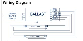
The wiring diagram that appears above is for the lamp type denoted by the asterisk  $(\ensuremath{^*})$
