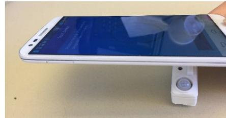
After programming successfully, a green check mark will appear on the screen. More sensors can be programmed with the same setting by pressing "Program EasySense again." Or press "Done" to finish configuration.
