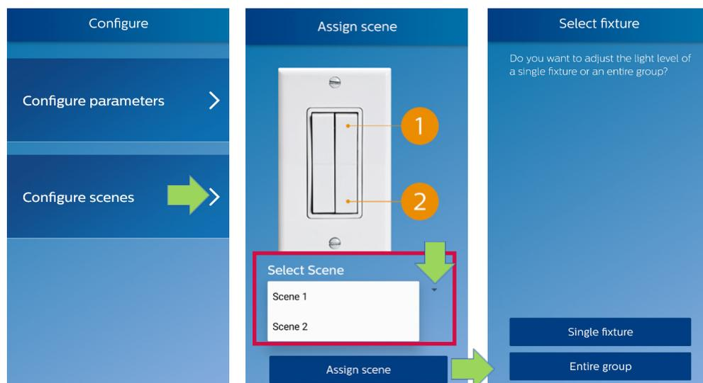
The scenes are selectable via the scene buttons of the switches associated either to fixture or an entire group.
