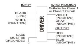
Input and output use lead- wires.
